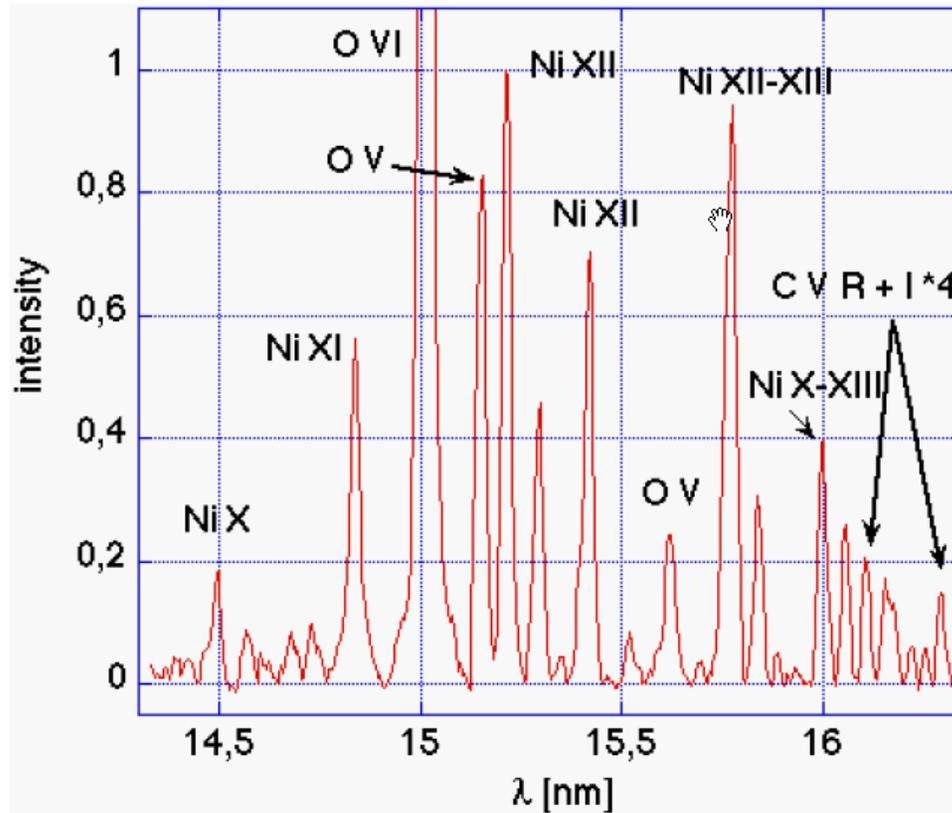
*Experimental and simulated M-shell nickel spectra in the 14.4–18.0 nm region from magnetic fusion devices*
