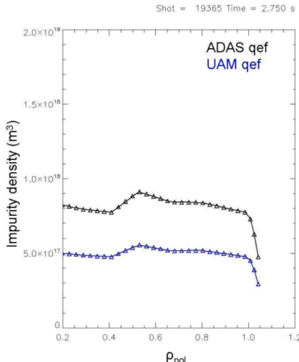
Radial density profile obtained from the fitting of calculated intensity for the transition to the experimental one using the CHEAP code in different shots in ASDEX-U.
