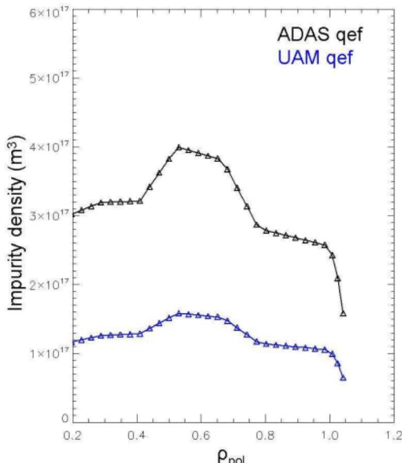
Radial density profile obtained from the fitting of calculated intensity for the transition to the experimental one using the CHEAP code in different shots in ASDEX-U.
