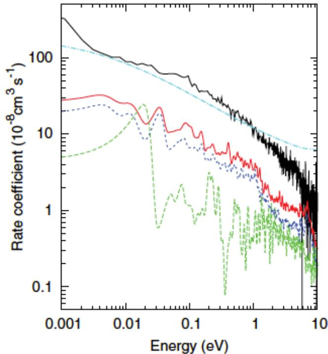
FIG. 5. (Color online)  $W^{20+}$  merged-beam DR rate coefficients: experiment [7] [upper solid (black) curve], partitioned total [dot-dashed (cyan) curve], IC total [lower solid (red) curve], LS total [long-dashed (green) curve], and IC  $4d \rightarrow 4f$  only [short-dashed (blue) curve].
