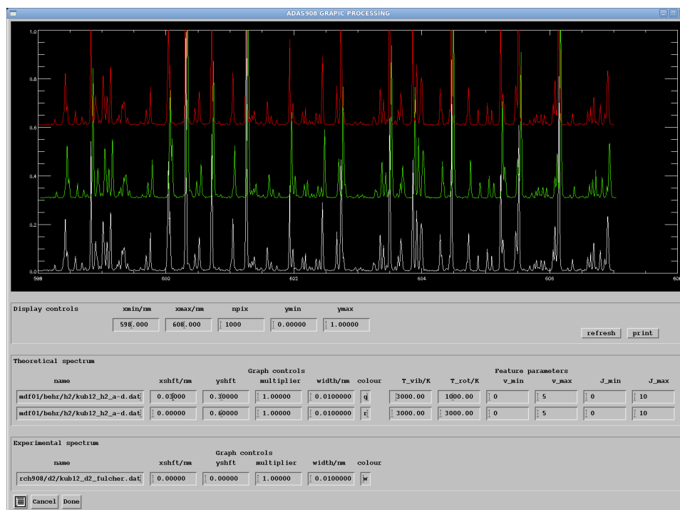
Figure 2.9: Illustration of spectral comparison and adjustment of spectra for identification. The widget is self adjusting dependent on how many theoretical and experimental spectra are to be compared.
